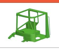
All-steel cab structure (FOPS and ROPS tested)
