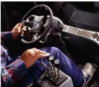
Hydraulic or electric servo control by levers.
