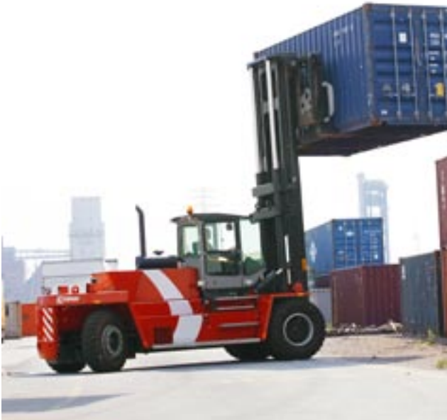
Handling of loaded 20' containers with forks.
