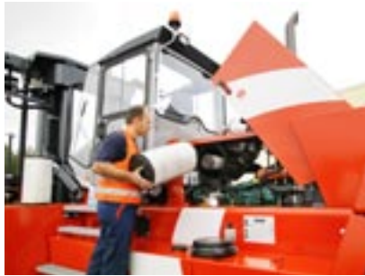
The air filter is easy accessible under the bonnett.
