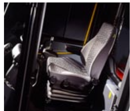
Driver's seat with mechanical or air assisted adjustments.
